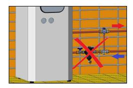
Upside-down and horizontal installation of the magnetic dirt separator MUST BE AVOIDED
